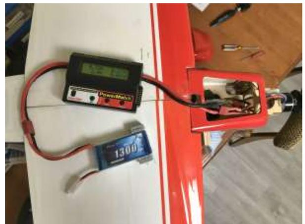
*Meter connected in series with the Lipo battery and ESC*
