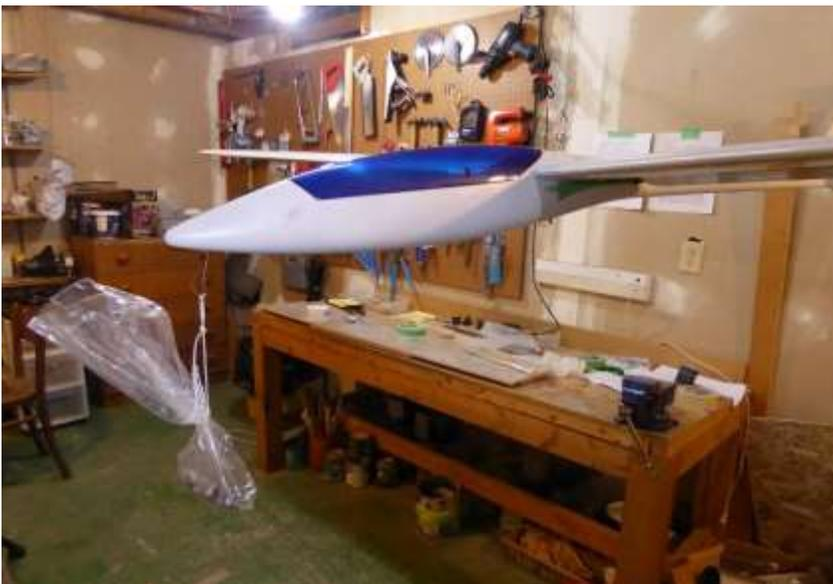
*Plane slung at balance point with required amount of lead ballast to be installed hanging on nose.*
