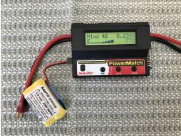
The meter can also be used to check remaining charge and voltage of NiCad & NiMH packs.
