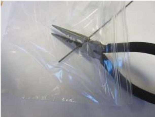
*How many times have you tried to cut off a piece of wire or carbon rod only to have the cut off piece go flying through the air, never to be found again! This is such a simple solution, try it out next time.*
