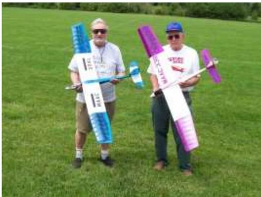
Roy Bourke holds a "**Spirit of Yesteryear, Talisman**" sailplane with the conventional tail (Vee and Tee also shown on plans). Roy has also modified the wing, making it straight and adding spoilers. The motor is a KD-A22-10S from Hobby King, Prop is a Graupner 9/7 folding, Battery is a 2 LiFePo4 1100 mAh cells in series and a 30 amp ESC. The covering is Ultracote Light. All up weight is 19 oz..
