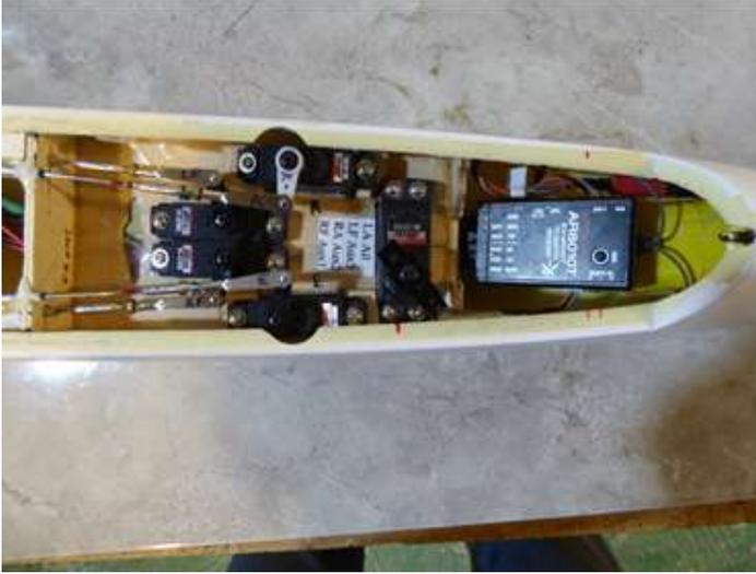
*The flap servos are at the rear, elevator and rudder at the side, tow release at the front*
