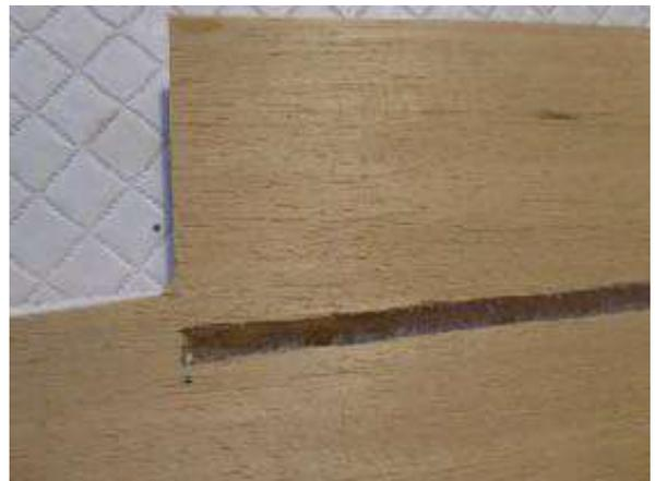
Flap 1st slot prior to balsa filling and cutting off the flap from the wing
