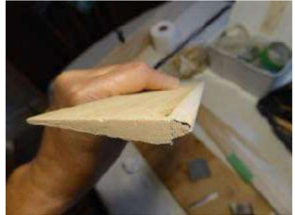
Flap leading edge protrusion that fits inside the 2nd slot
