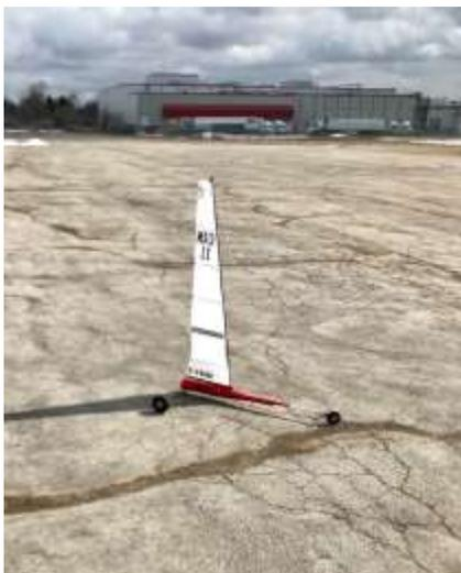
Sailing a land yacht is **not** like sailing a boat on wheels but more akin to flying a sailplane. It's all to do with the "*apparent wind*". Due to their design and light construction, these wee beasts can go 2 to 3 times the speed of the wind!! Most of the time the sail is close hauled even when going downwind! It's really a different form of "sailing".
