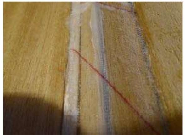
Flap peel-ply fabric (cut on a 45° bias) hinge
