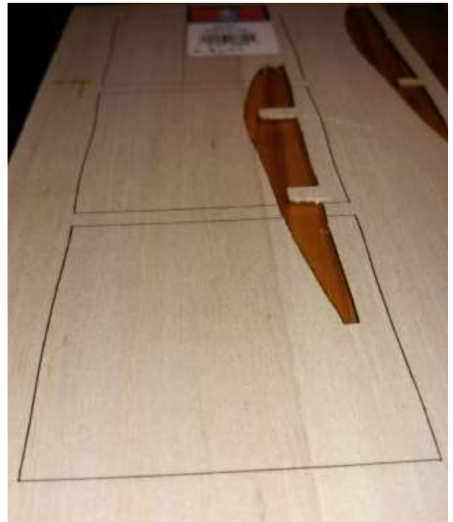
Less-than-straight cuts due to wobbly wheels.
