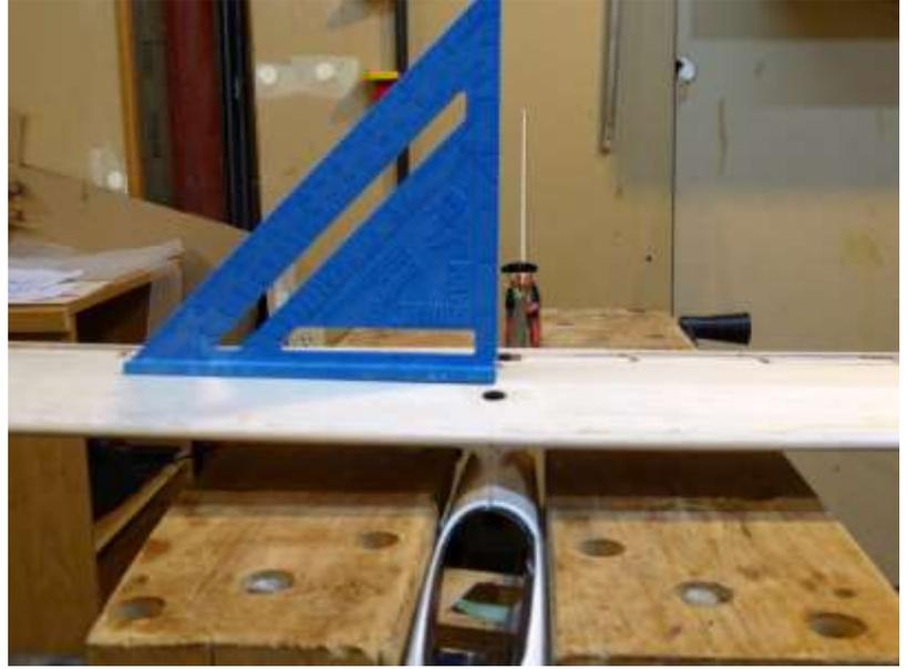
Squaring the vertical stab/rudder before gluing to the boom
