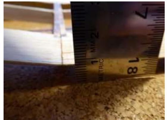
Checking washout at the mid to tip wing
