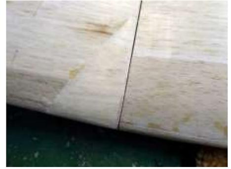
Correcting LE mismatch at centre to mid wing joint
