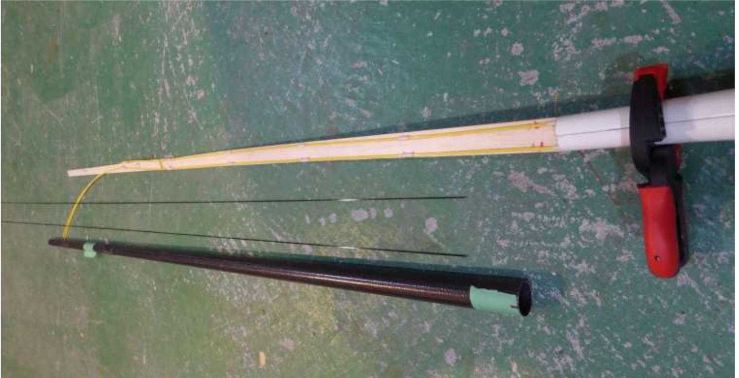
Pushrod tube restraint in the boom before assembly
