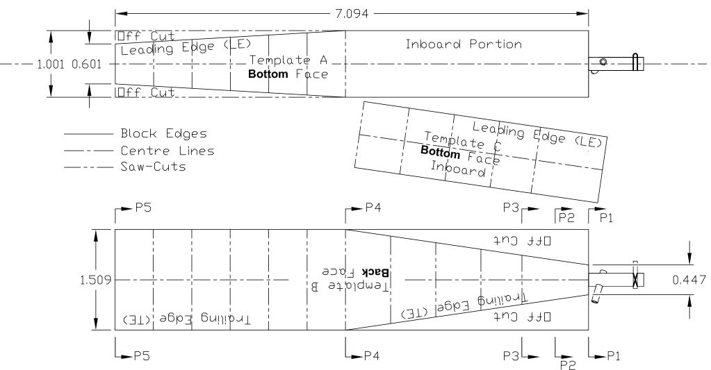
Templates for 17.25 Dia. x 21.6 Pitch Propeller
